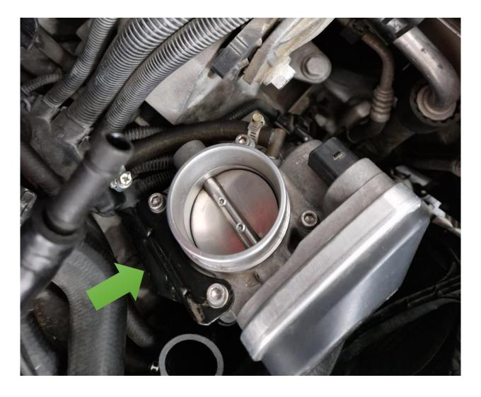
9. Install the fourth and final bolt. You will have to push the bracket towards the throttle body. Once the bolt is through, torque in place the throttle body bracket.
