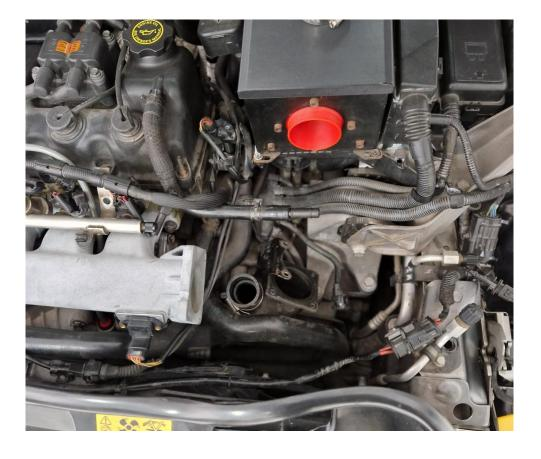
5. Remove the throttle body and the vacuum line that is connected to it. Then remove the vacuum line from the original charge pipe.
