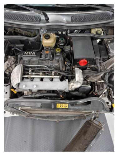
3. Remove the intercooler diverter, the intercooler and the silicone hose that connects the throttle body and the airbox.
