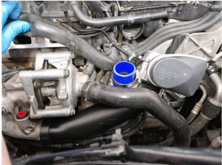
11. Make sure the charge pipe is fitted as in the photos.Then proceed on installing the crash bar spacers.For this step you will also have to remove part number 7 (see diagram below).
