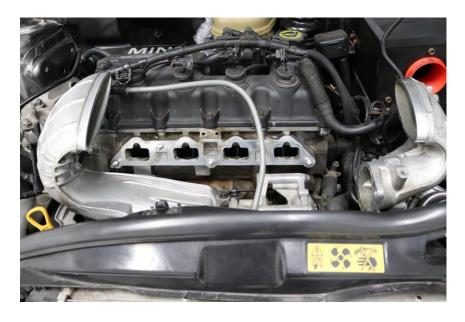
1. Disconnect the battery, remove the intercooler and original intake manifold.
