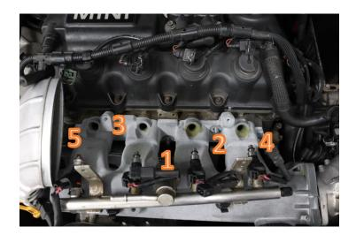
4. Connect the fuel rail vacuum take-off to the intake manifold. Do not bolt the fuel rail yet. Install the intake manifold. Tight the bolts following the numbers in the picture above. Use medium strength threadlocker to all studs. For this step you will reuse the original nuts.
