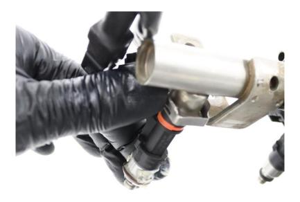
3. Remove the original injectors orings and install the orings that are provided with the kit. Apply silicone grease as in previous step.
